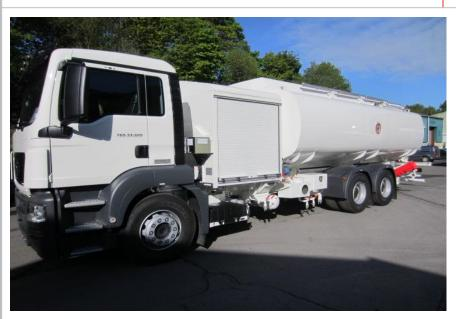
A 25,000L useable capacity rigid refueller mounted on a 6x2 chassis. The refueller is equipped with 1 x underwing and 1 x overwing hose, single meter and filter water separator or an optional filter monitor. Options include a weatherproof cabinet. The refueller conforms to latest European Standards EN12312-5 and JIG1 Issue 12 requirements.
